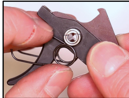
Step 28: Re-Attach your Trigger Return Spring. Make sure both loops of the Spring Seat on the ends of the Bushing.
