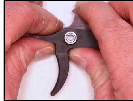
Step 28: Re-Attach your Trigger Return Spring. Make sure both loops of the Spring Seat on the ends of the Bushing.
