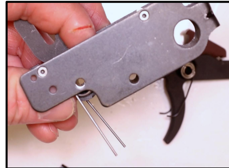
Step 32: Drop your Hammer into position in the Trigger Housing.
