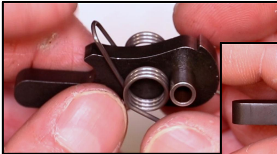
Step 30: Grab your New Hammer Spring and get each loop to Grab.
